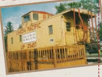
The design features a high, centered cupola which makes UP steel cabooses one of the most recognizable cabooses in North America. The caboose is equipped
